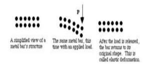
Dislocations move easily in metals, due to the delocalized bonding, but do not move easily in ceramics. This largely explains why metals are ductile, while ceramics are brittle.
