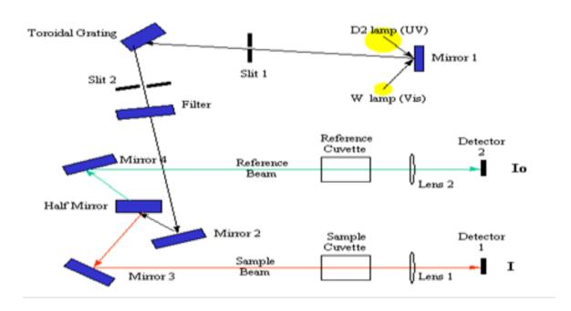
The functioning of this instrument is relatively straight forward. A beam of light from a visible or UV light source is separated into its component wavelengths by a prism or diffraction grating. Each monochromatic beam in turn is split into two equal beams by a half-mirrored device.
