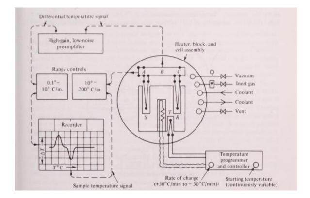
Typical DTA equipment is illustrated in Fig. The furnace contains a sample block with identical and symmetrically located chambers Each chamber contains a cen- tered thermocouple. The sample is placed in one chamber and a reference material, such as a AlgO,, is placed in the other chamber. The furnace and sample block temperature are then increased at a linear rate, most often 5 to 12°C/min, either by increasing the volt age through the heater element by a motor-
