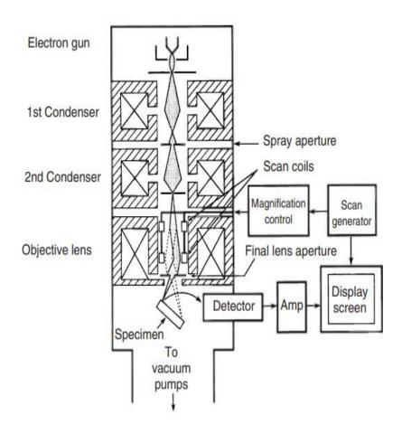
These collected electrons produce scintillation on photo multiplier tube (detector) and are converted into electrical signals. These signals are amplified by
