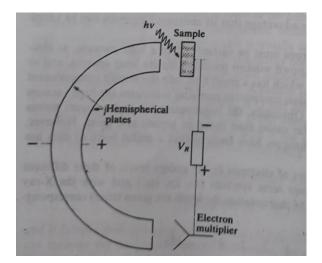
The resulting electron current, measured by an electron multiplier, indicates the number of electrons ejected from the surface with that kinetic energy.  $E_u$  can be systematically varied by changing the retarding voltage (V) applied to the analyzer. Thus a photoelectron spectrum is a plot of the number of electrons emitted against their kinetic energy.
