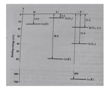
Figure shows the binding energies of electrons in the energy levels of three different dements. The levels are labeled with their term symbols (13, 2p, etc.) and with the X-ray rotation which is sometimes used in PES. In this notation the levels are given letters corresponding to their shell:
