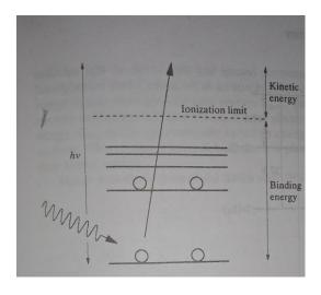
Electrons can be ejected from either the core or the valence levels of the atom, depending on the energy of the exciting radiation, and their kinetic energies are characteristic of the atom from which they have been emitted. If the atom is part of a molecule, the energy of its valence electrons (and, to a much lesser extent, its core electrons) will be modified by the bonding but are nonetheless characteristic of the orbital in question
