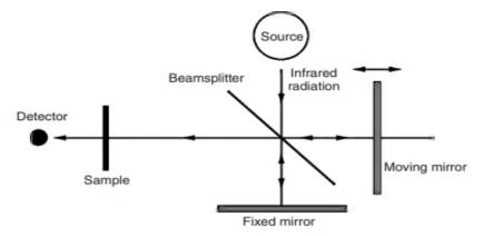
Fourier transformation is necessary to convert an interferogram into an infrared spectrum, which is a plot of the light intensity versus wave number. The Fourier transform is based on a fact that any mathematical function can be expressed as a sum of sinusoidal waves. All the information of wave intensity as a function of wavelength is included in the sum of sinusoidal waves.
